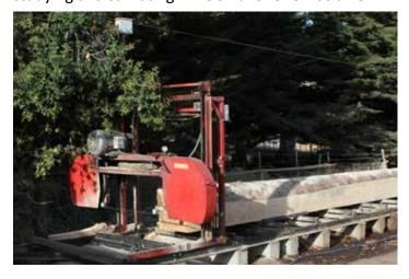
wide Linn horizontal bandsaw driven by a three-phase electric motor and appeared to be propelled through the cut by a hand driven winch. If that saw did not offer enough capacity, the monster next to it would almost certainly fill the bill. This was a chain saw mill, with a 12' bar and 10' net cut width. The bar was
